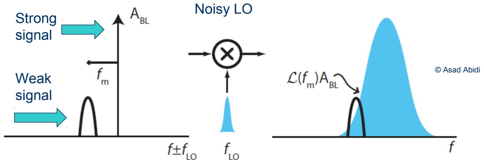
Noisy local oscillator (LO) transfers its noise to the strong out-of-passband signal and on top of the weak signal we are trying to copy.
